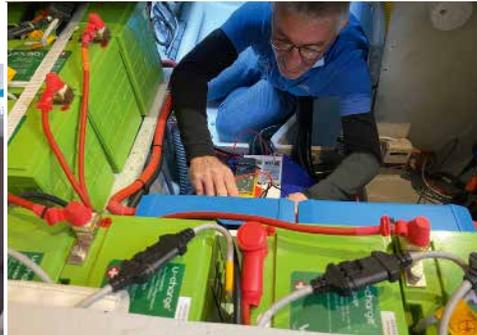
Testing Oceanvolt's output to the two banks of 28kWh batteries
