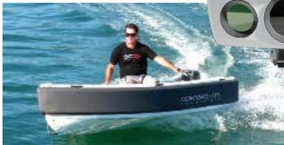
Above: OCT tender with electric outboard. Inset above: the OSCAR camera detects floating objects using artificial intelligence
